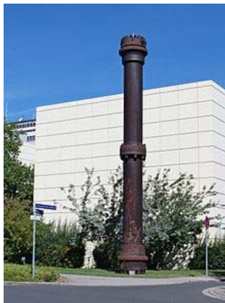
This high-pressure reactor was built in 1921 by BASF in Ludwigshafen and was re-erected on the premises of the University of Karlsruhe in Germany.
